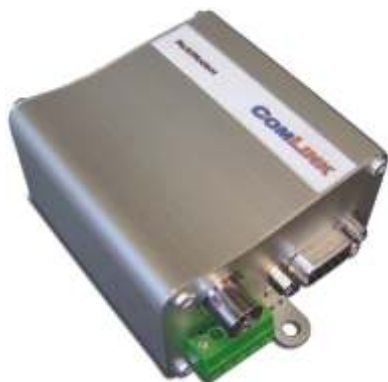
MultiModem i robust aluminiumkapsling
